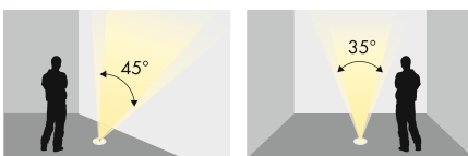
Asymmetrische Linse 45°/35° / Asymmetrical lens 45°/35°
